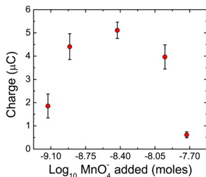
**Figure 2.** Optimization of the electrochemical signal in the *o*Slip. Plot of charge under the ASV peak as a function of the number of moles of  $\text{MnO}_4^-$  added. The number of moles of Ag was kept constant. The error bars represent the standard deviation for three different measurements.
