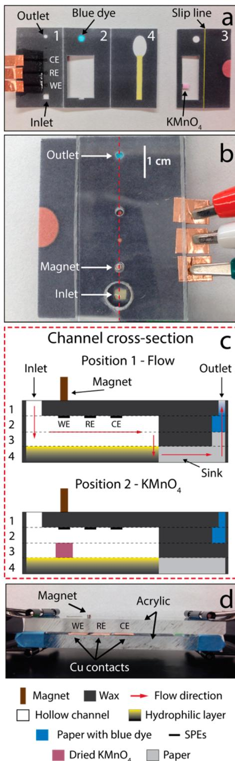
by adding 50.0  $\mu\text{L}$  of PBCl buffer containing different concentrations of the model analyte to the Inlet while the Slip layer is in position 1 (Scheme 1c). In this configuration, the sample flows horizontally across the hollow channel and the model analyte is concentrated at the working electrode by the magnetic field (first preconcentration step, Scheme 2a, also see blue-border inset). The PBCl buffer and any other components
