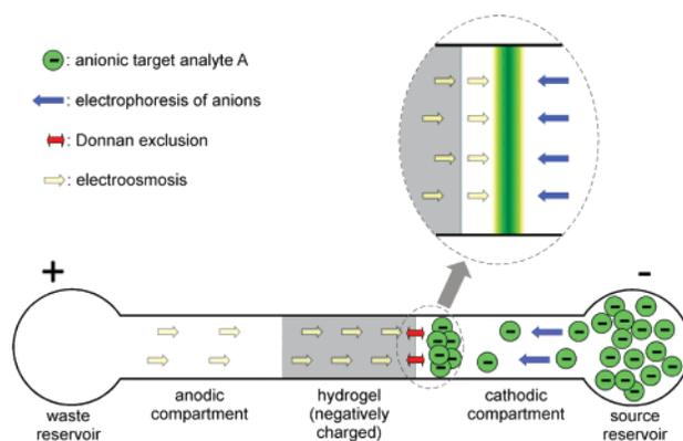
**Figure 1.** Schematic illustration of transport processes in the microfluidic device containing an immobilized, negatively charged hydrogel microplug with a mean pore size comparable to the electrical double layer thickness.
