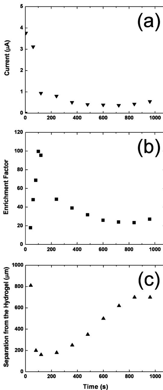
**Figure 4.** (a) Electrical current through the microfluidic device, (b) enrichment factors, and (c) displacement of the analyte enrichment zone as a function of time in the cathodic microchannel compartment. Applied potential bias, 100 V (forward). The enrichment factors correspond to the respective peak heights in the fluorescence intensity profiles shown in Figure 3c.
