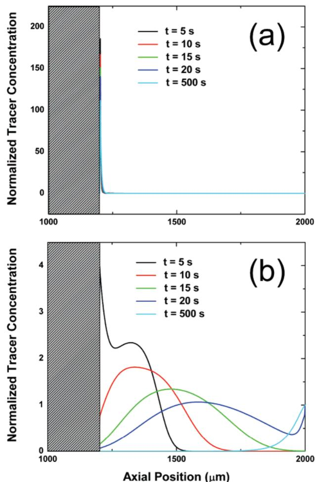
**Figure 7.** Transient tracer profiles in the cathodic microchannel compartment which covers the distance from  $x = 1200$   $\mu\text{m}$  to  $x = 2000$   $\mu\text{m}$  (cf. Figure 2b) for  $E_{\text{ext}} = 11.1$  kV/m, (a) without and (b) with EOF in the device. The EOF correction factor is assumed to be 0.1.
