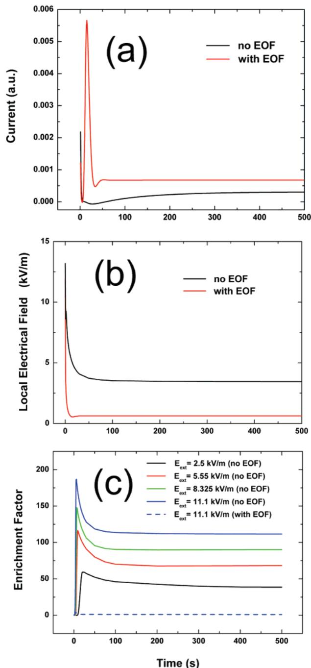
**Figure 6.** (a) Current flowing through the device after application of  $E_{\text{ext}} = 11.1$  kV/m without and with EOF, (b) corresponding transient behavior of local electrical field at the cathodic membrane–solution interface, and (c) transient enrichment factor as a function of the applied electrical field strength. The EOF correction factor is assumed to be 0.1.
