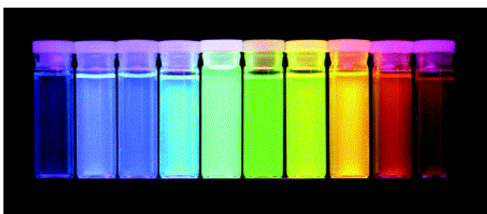
Figure 2. Ten distinguishable emission colors of ZnS-capped CdSe QDs excited with a near-UV lamp. From left to right (blue to red), the emission maxima are located at 443, 473, 481, 500, 518, 543, 565, 587, 610, and 655 nm.
