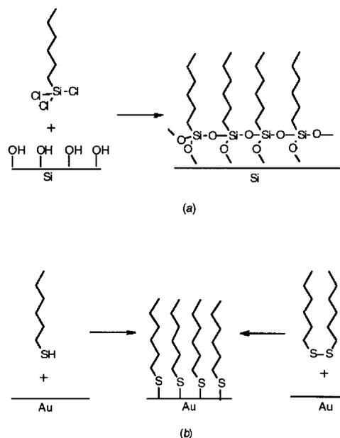
Fig. 3. Formation of trichlorosilane-SiO<sub>2</sub> (a) and gold-thiol (b) monolayers.
