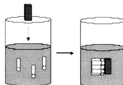
Fig. 1. Exposure of a substrate to a surfactant solution leads to formation of a SAM. The principal driving force for SAM formation is the affinity of surfactant head groups for the surface of the support.
